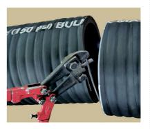
Cut the steel helix wire. The wire must not protrude past the end of the hose
