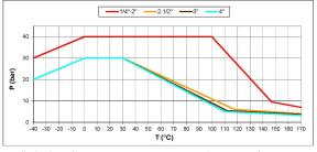
AS4617 limitations for GAS: 2100 Kpa up to 2" and 1500 Kpa from 2. 1/2" to 4" rated working pressure and  $0^{\circ}\text{C}$  +60°C temperature
